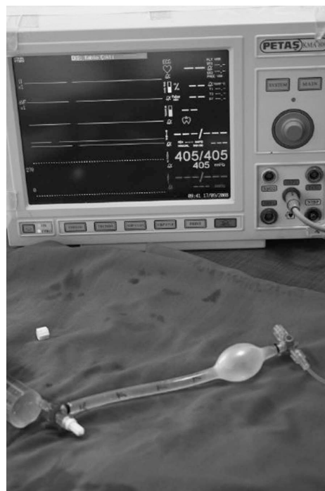
Dikmengil-Yilgör TF-1 vascular graft kept its shape until 405 mmHg and above this value an aneurism of 20.4 mm diameter occurred
